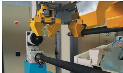
Because even a 1mm variation in wall thickness can impact hose life by 25%, every hose is precision machined to ensure repeatable performance.
