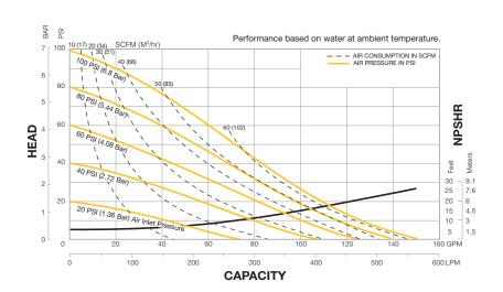
MAX CAPACITY 150 GPM (568 LPM)
